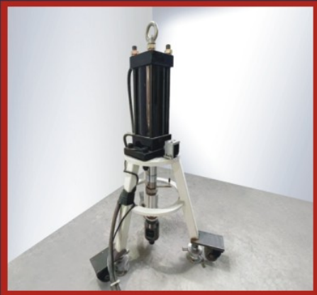
Pull out in concrete
