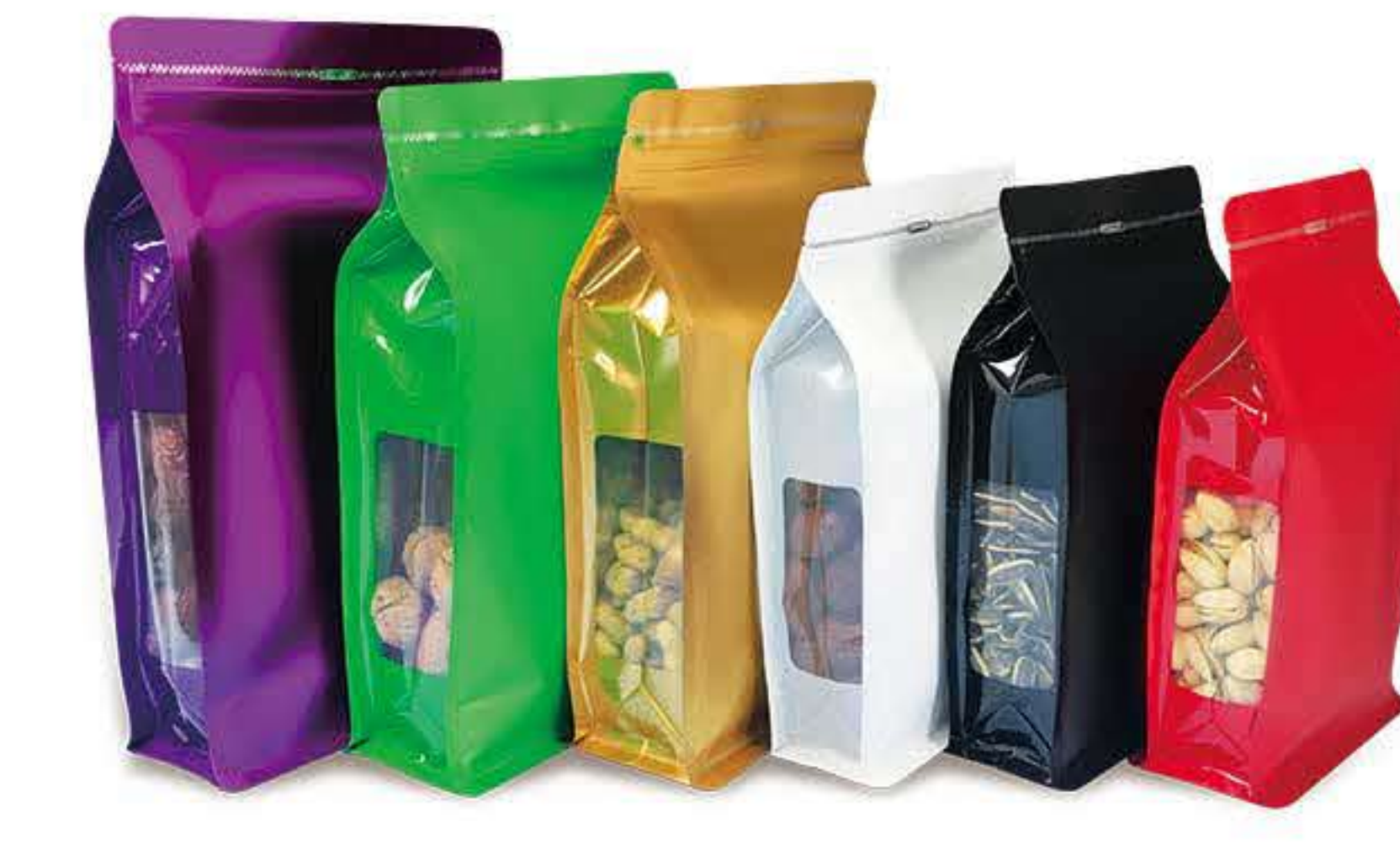
Eight side seal pouch with zipper (Matt outside) Thickness(one side):130mic Material: MOPP/VMPET/PE 14*24+3.5cm*2 16*24+3.5cm*2 18*28+4cm*2 20*30+4cm*2
