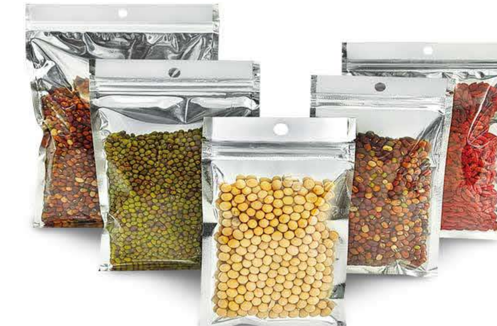
3 side seal pouch with zipper (one side transparent, one side foil Glossy outside) Thickness(one side):80mic Material: Front: PET/ PET/ CPP Back: PET/ VMPET/ CPP
